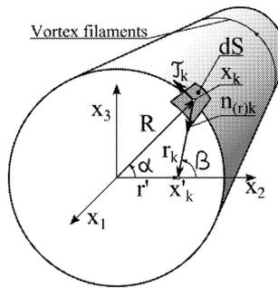
Fig.3: Circular vortex filaments aligned in the infinite length vortex tube
