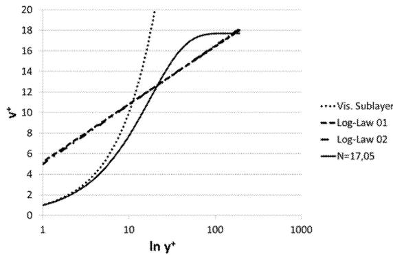
Fig.5: The Comparison of velocity profile near the wall with the log-law
