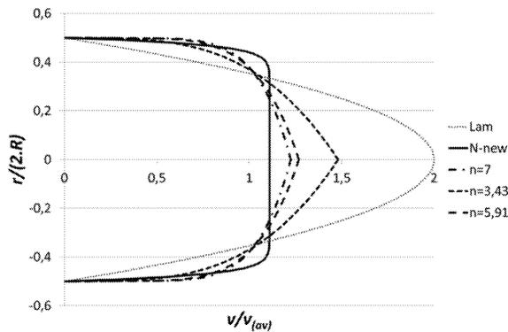
Fig.4: The comparison of velocity profiles
