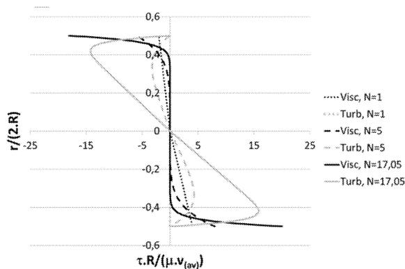
Fig.6: The viscosity and turbulent shear stresses
